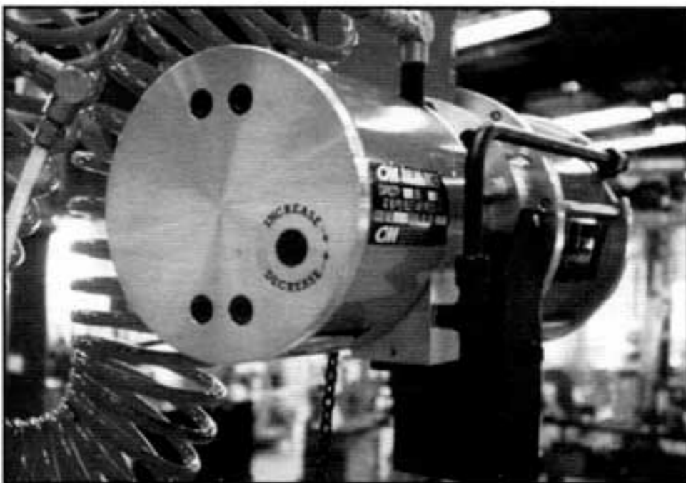
Figure 8. CM Max balancer with single load balancing control
